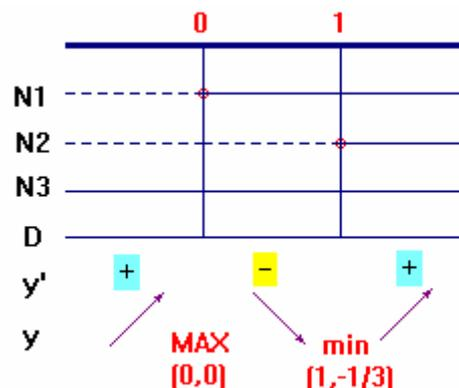
□ **Derivata seconda**  $y = \frac{x^3 - 2x^2}{x^2 + x + 1}$   $y' = \frac{x^4 + 2x^3 + x^2 - 4x}{(x^2 + x + 1)^2}$
