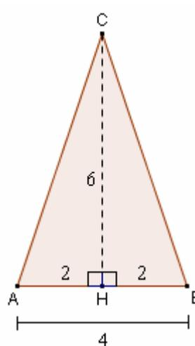
$$\begin{aligned} CA &= \sqrt{CH^2 + \left(\frac{AB}{2}\right)^2} = \\ &= \sqrt{6^2 + 2^2} = \sqrt{36+4} = \\ &= \sqrt{40} = 2\sqrt{10} \text{ cm} \end{aligned}$$
